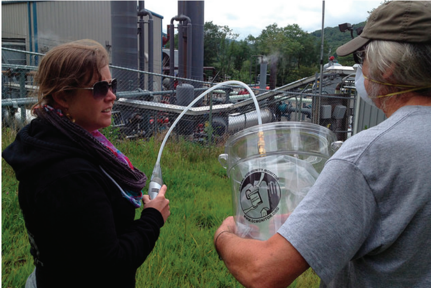
Volunteers using a “bucket” for sampling air near an industrial plant. Photo Credit: Global Community Monitor
