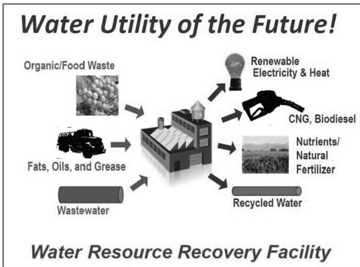
Figure 1. Co-Digestion of Food Wastes and Resource Recovery at WRRFs (Reprinted with permission by the Water Environment Federation)
