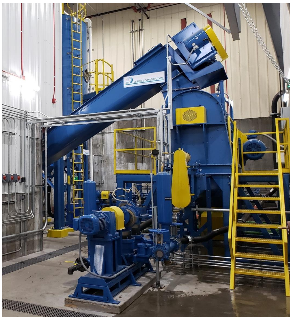
Figure 1. Scott Equipment THOR Turbo Separator in the Oneida-Herkimer Solid Waste Authority SSO Preprocessing Facility in the Eastern Transfer Station. Source: OHSWA.
