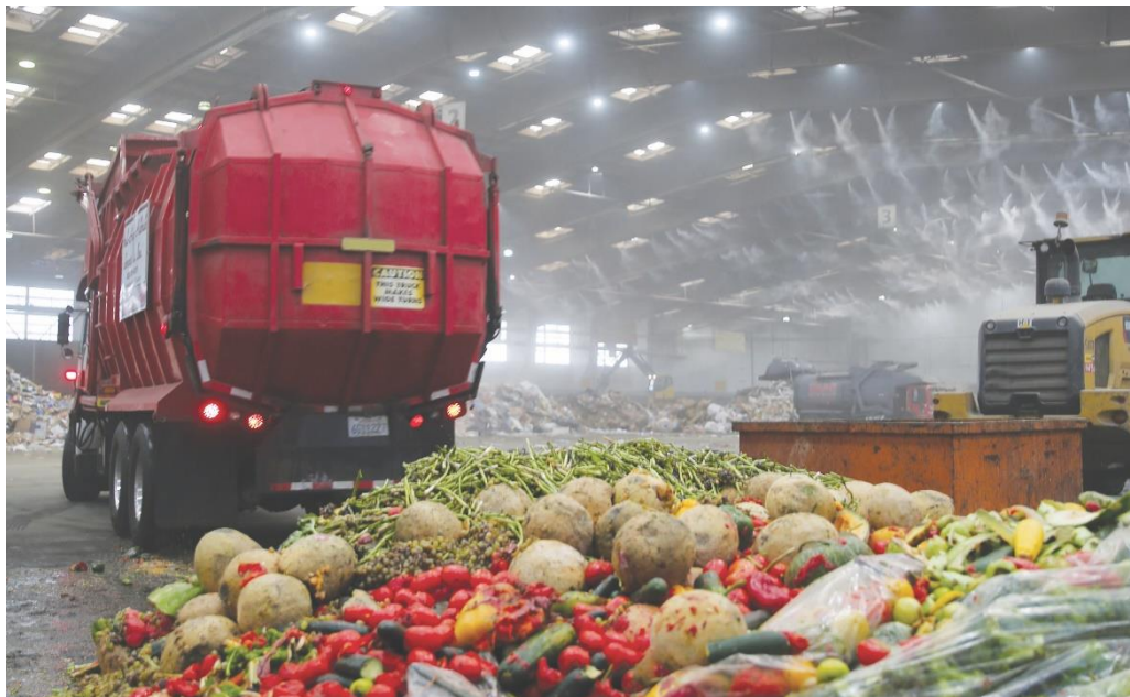
Figure 4. Truck unloading food scraps on tipping floor at Puente Hills MRF. Source: LACSD.
