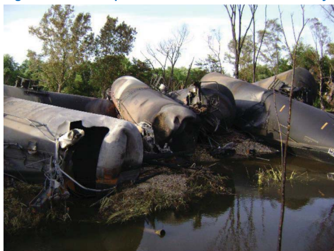
Figure 19 – Close up of DOT-111 Tanks Cars after Cherry Valley, Illinois Derailment and Fire 64
