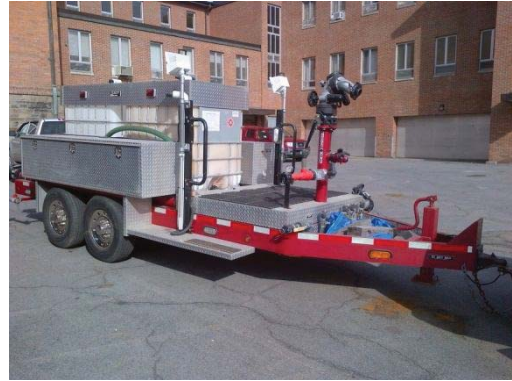
Figure 26 – Firefighting Foam Trailer
