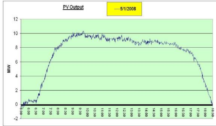
Figure 2.11: PV plant output on a sunny day (Sampling time 10 seconds)
