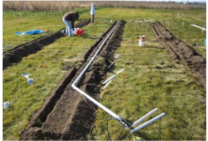
Field staff installing suction tube lysimeters. Lysimeters collect water that escapes below the root zone of growing crops. Collected water will be analyzed for nitrate-nitrogen.
